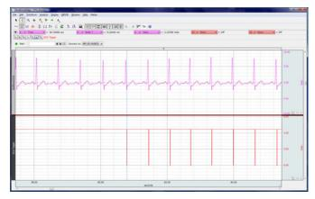
In the figure at left, a DA100C amplifier captures the respiration signal using a TSD110-MRI transducer on Channel 1, and an ECG100C amplifier captures the ECG signal on Channel 2. These signals are captured to the MP150 and the UIM100C and provide analog outputs of the signals via CBL102 cables Labeled cables are provided with the DTU200/300 system to ease setup.
