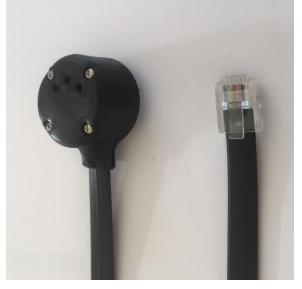
The TSD303 Barometric Pressure Transducer measures atmospheric barometric pressure in a range of 0 to 15 psi. It may be used in various applications where corrections for ambient environmental barometric pressure is required.
