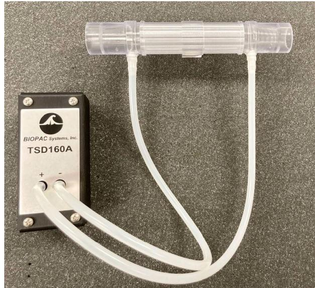
The TSD157B-MRI laminar flow transducer ( $\pm 120$  LPM) is suitable for precision ventilator bidirectional airflow measurements or resting airflow measures in fMRI. It consists of flow head RX157B + pressure transducer TSD160A + Tubing. Available with 20 m tubing for MRI use or 1 m tubing for non-MRI use (option TSD157B-MRI-01). Tubing presses over the barbs on the flow head and transducer and should be cut to fit for max separation, typically 10 m for MRI or 0.5 m for non-MRI.
