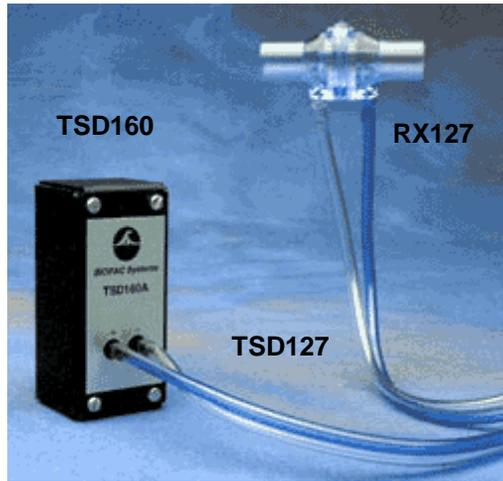
The TSD127 can perform a variety of pulmonary measurements relating to airflow, lung volume and expired gas analysis. The TSD127 is intended for animal and human use and consists of a pneumotach airflow head (RX127) coupled to a precision, highly sensitive, differential pressure transducer (TSD160A). The TSD127 will connect directly to a breathing circuit or plethysmogram chamber. The detachable flow head (RX127) makes cleaning and sterilization easy.
