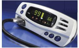
The sensor cable material is a light conducting glass bundle made up of premium achromatic glass. There is no conductive cable running through the sensor cable except what is encased in the control unit side DB9 connector. The photo detector and LED are in that end and connected to the respective fiber optic ends.
