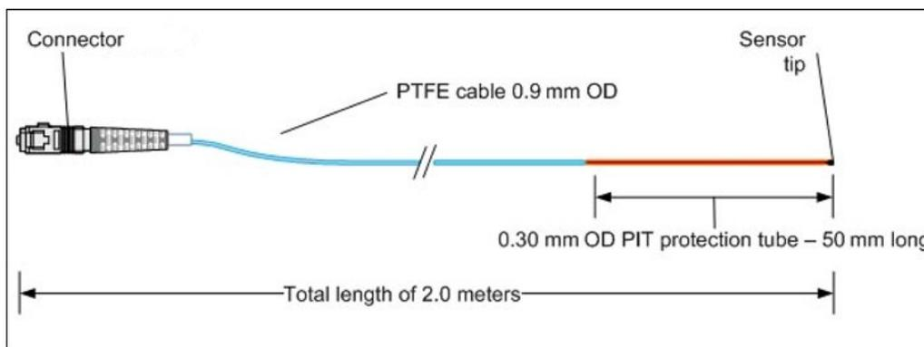
The TSD280A and TSD282A are micro pressure sensors that connect directly to the MPMS200A unit.
