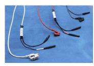
The LEAD110 Series, for use with disposable and other snap connector electrodes, are pinch leads for easy connection between the EL500-series snap electrodes and any BIOPAC biopotential amplifier or the GND terminal on the back of the UIM100C. Leads are 1.9 mm in diameter and terminate in standard 1.5 mm Touchproof connector and connect to BIOPAC modules or to a Modular Extension Cable (MEC series).
