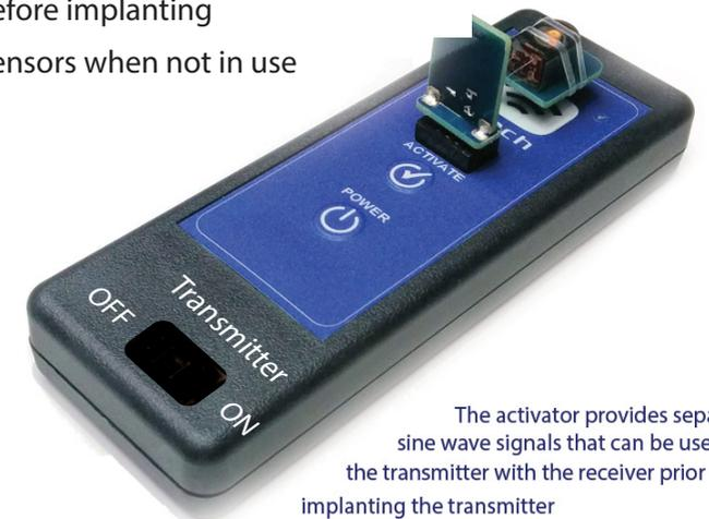
The activator provides separate sine wave signals that can be used to test the transmitter with the receiver prior to implanting the transmitter
