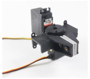
This Robot Gripper with 2 x Robot Servos is used for the EMG-Controlled Robotic Arm created with BSL *PRO* Lesson Set H40 (10 labs).
