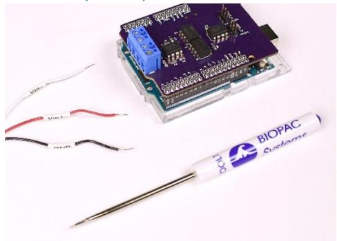
This Development Board with Shield is required for the overall system test in Lab 10 of the <a href="H40 EMG-Controlled Robotic Arm Lesson Set">H40 EMG-Controlled Robotic Arm Lesson Set</a>; a script and instructions for running the BSL-DEV-S are included in the lesson journal and lab protocol. The Development Board converts both EMG analog signals to PWM (pulse width modulation) digital signal, which drives each Servo motor. The shield provides optical isolation.
