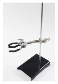
This lab ring and clampstand can be used when building the EMG-powered robotic arm in the BSL PRO H40 Lesson Set. The base of the robotic arm consists of one lab ring stand and clamp, which holds two servo motors and a gripper (BSL-GRIPKIT) in place. The stand is a cast iron support ring stand with acid resistant finish. The platform is 20 cm x 30 cm (5" x 8") and the rod is 51 cm (20") tall. The clamp is a 3-prong finger style rubbercoated laboratory stand clip made of alloy steel.
