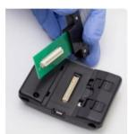
Connecting B-Alert Universal EEG Strips to the adapter and then the adapter to the headset.
