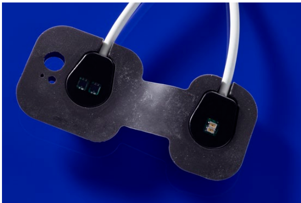
moorVMS-NIRS Probe Heads – emitter and detector.
