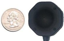
The TSD250A is a sensitive accelerometer (32.64 mm diameter) that uses advanced signal analysis algorithms to monitor small muscle vibrations that occur when a muscle is activated. This transducer is optimized for assessing voluntary muscle effort and includes band-pass filtering for eliminating most motion artifacts including physiologic tremor.
