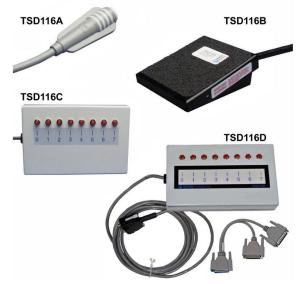
**TSD116D** — eight-channel marker box that connects to the 25-pin connector on the back of the STP100C/D only. Ships with a Y-splitter cable to allow the parallel port to be connected to a stimulation presentation system. TSD116D terminates in a 25-pin DSub pass-through connector with the ground line (pin 18) of the box and each of the switches wired to the appropriate digital input pin of the DSub connector (pin 2 through 9).
