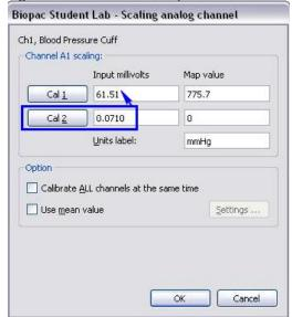
Adding 0.071 to the initial value of 61.44 results in an adjusted **CAL 1** value of 61.51 mV. (Your result may vary slightly from the example).
