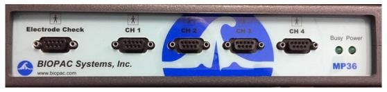
The front panel of the MP36R has an electrode check port, four analog input ports, and two status indicators.
