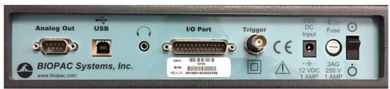
The back panel of the MP36R has an analog output port, a USB port, an I/O Port, a Trigger Port, a DC input, a fuse holder, and a power switch, and the unit's serial number.
