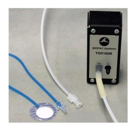
The transducer assembly includes a self-inflating pressure sensing pad connected to tubing terminated in a Luer male connector to interface additional tubing included for connection to the transducer. The pressure pad can be used many times, but may eventually need to be replaced if the sensor is damaged with rough or prolonged use.
