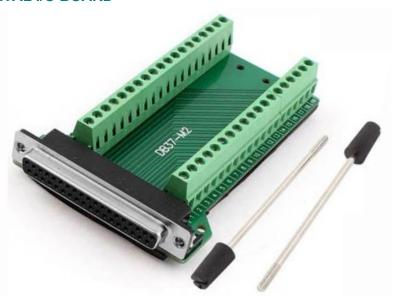
The STP-IO allows for access to the isolated digital input and output lines of the STP100D module. This digital breakout board connects directly to the 37-pin connector on the STP100D, providing access to digital channels 0-7 for digital output and digital channels 8-15 for digital input.
