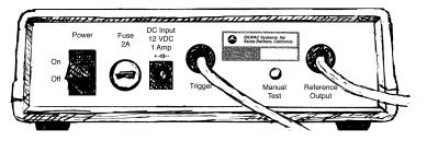
Power Rocker switch for turning the STM200 power ON and OFF.
