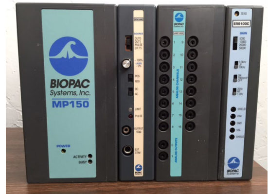
STM100C connection to MP device, UIM100C and ERS100C
