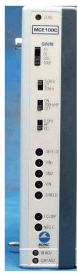
The MCE100C is an extremely high input impedance, low noise, differential amplifier that accurately amplifies signals derived from mini and microelectrodes. Mini and micro electrodes are characterized by small surface contact areas that result in high electrode to tissue contact impedance. A number of selectable options make the amplifier module useful for general-purpose recording of cortical, muscle and nerve action/resting potentials.
