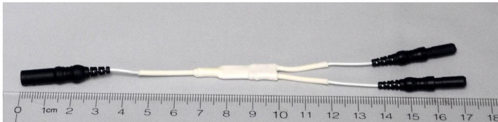
This “Y” cable is functionally identical to the JUMP100C, but designed for use in the MRI environment when referencing two or more amplifier inputs to a single electrode input. Primarily used for recording biopotential measurements for EEG, ECG or EMG in the MRI. Two 1.5 mm Touchproof female inputs to one 1.5 mm Touchproof male input, cable length 10 cm.
