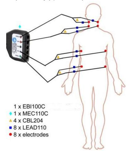
**NOTE:** The EBI100C measures bioimpedance in terms of both magnitude and phase as a function of frequency (12.5, 25, 50, and 100 kHz). The choice of interfacing cables will impact both magnitude and phase readings. The impacts will be larger as the frequency of the source current increases. To obtain accurate measures at any frequency, calibrate the measurement for magnitude and phase after the interface cabling infrastructure is stabilized. (See EBI100C Calibration steps on page 4.)
