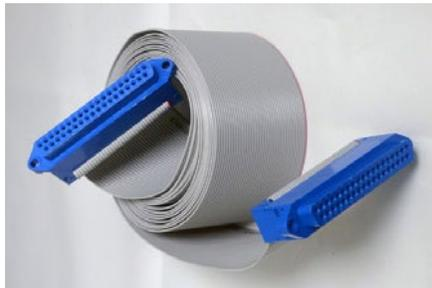
**CBL110C** DB25 M/F Ribbon Cable. Use this 3-meter ribbon cable to send digital I/O info to the STP100D Isolated Digital Interface to interface visual presentation systems that use a computer's parallel printer port (E-Prime, DirectRT, MediaLab, Inquisit, etc.) with an MP1xx System. Pins 18 and 25 are GND.
